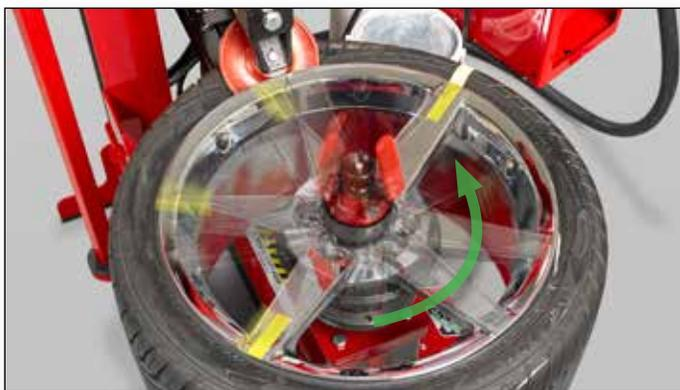
The Maverick™ tire changer's bead rollers allow spinning of tire on rim, helping match-mount stiffest point on tire to low spot on rim.
