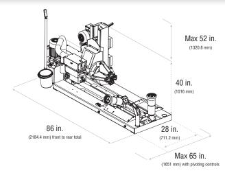
The TCX635 is designed to service truck-type tires with angled bead seats. Passenger car and light-truck tires cannot be serviced on this changer even if they are in the listed clamping range.
