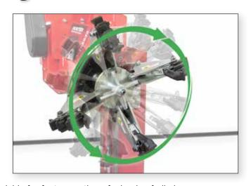
The innovative tulip-style clamp expands and contracts quickly for fast mounting of wheels of all sizes.
