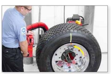
When combining ForceMatch® wheel balancer (left) with a heavy-duty tire changer (right), their match-mounting capability achieves the smoothest possible ride.
