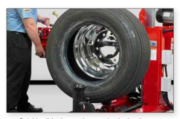
Quickly slide the carriage and spin the tire, rolling both beads off of the rim. It's that easy.
