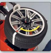
The bead rollers safely hold the tire stationary while the rim is rotated to complete match-mounting.
